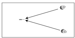
Figure 11b - Placement for Stereo Pair
